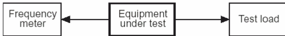
Figure 5.1.1.10: Measurement diagram for signal transmission rate (clock frequency error)
